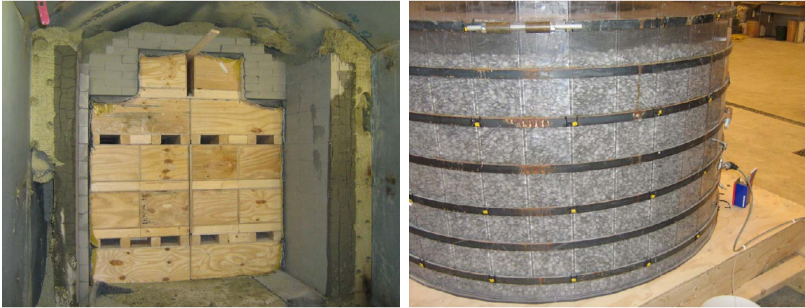
Figure 5-1. Piping and erosion test. Left: Halve scale backfilling test. Right: Buffer test.
