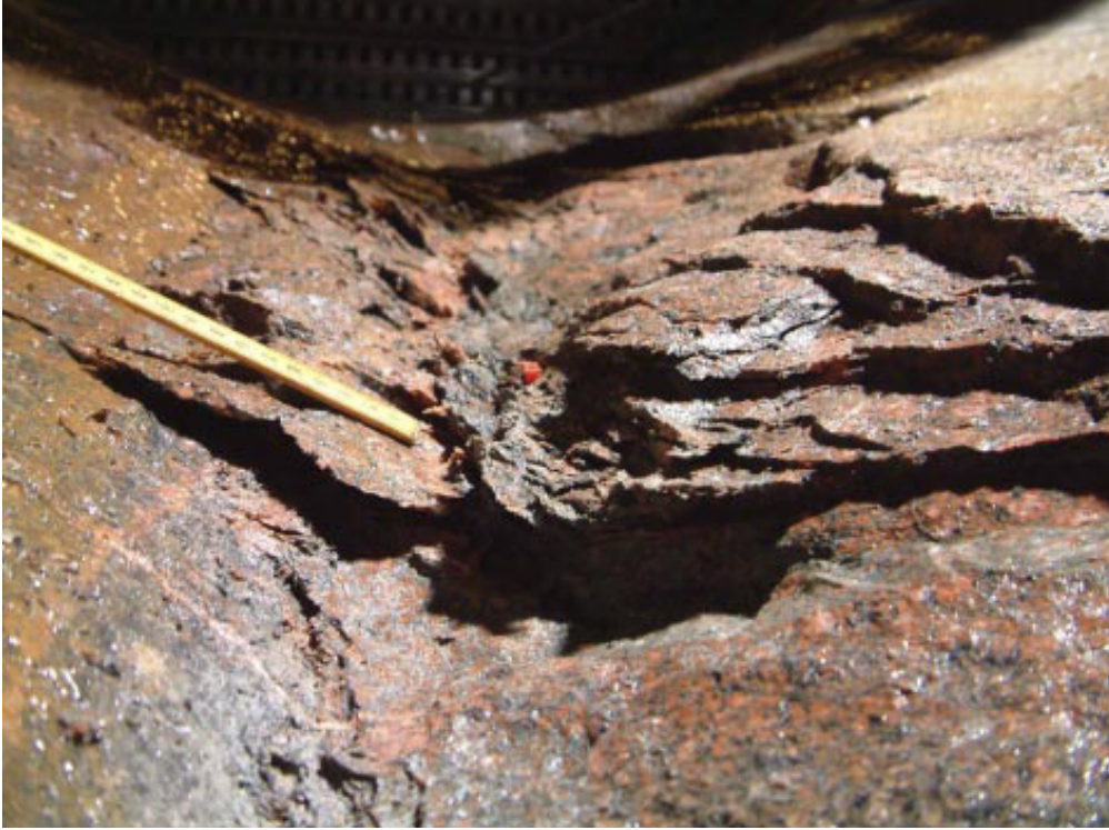
Figure 2-2. Cross section through spalled zone in the Pillar Stability Experiment (Apse) /Andersson 2007/.
