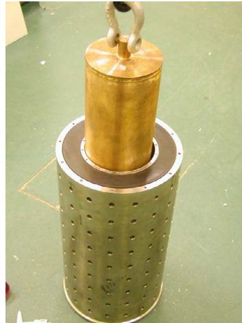
Miniature canister with support cage
