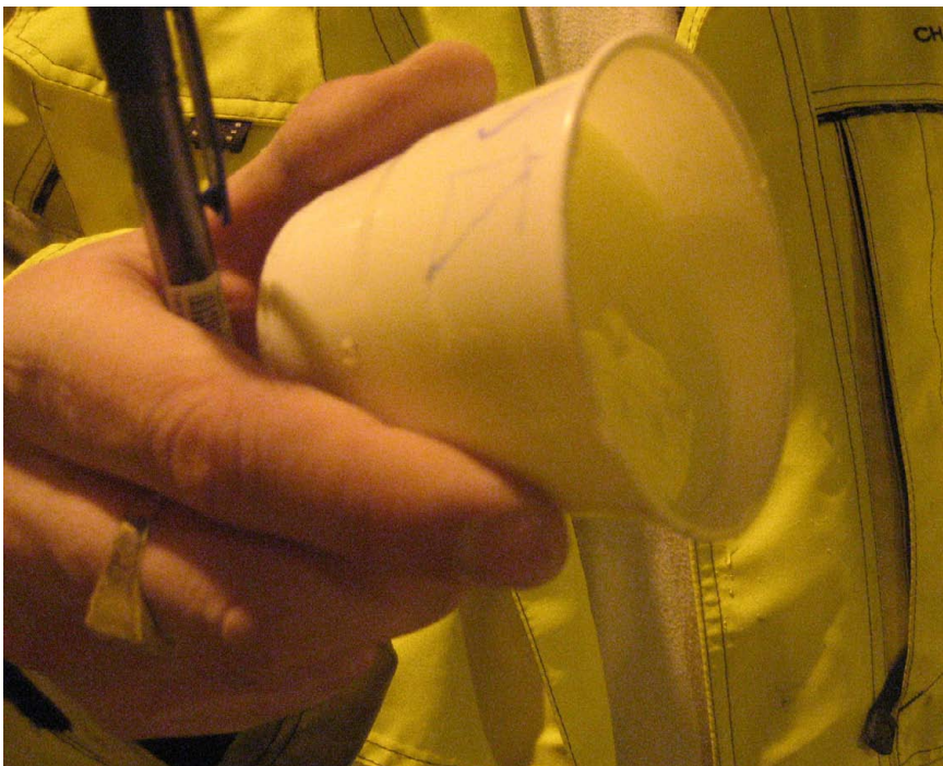
Figure 4-2. Silica sol – control of gelling time (photo: Ann Emmelin).
